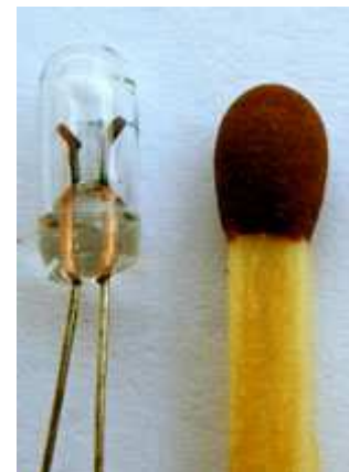
Fig. 3.4.2 Typical T1 Miniature Filament Lamp Compared With a Match Head
